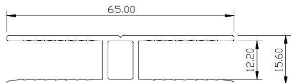
AA7660 JOINER MASS: 0.663 Kg/m AP: 274.48 mm CCD : 67
